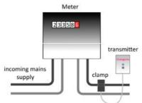
You will need to attach the clamp to the insulated live-feed cable between your electricity meter and your consumer unit. This cable is usually on the right hand side of the meter (as in the diagram). You can also attach to the incoming live supply on the left hand side of the meter if more convenient.
