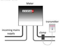
You will need to attach the clamp to the insulated live-feed cable between your electricity meter and your consumer unit. This cable is usually on the right hand side of the meter (as in the diagram). You can also attach to the incoming live supply on the left hand side of the meter if more convenient.
