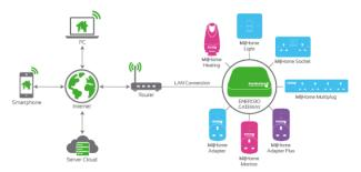
The Monitor adapter is part of the MiHome home automation range. The Monitor adapter allows you to monitor the power being used by an attached appliance. It links to the MiHome Gateway which provides the communications between your adapter and the internet.
