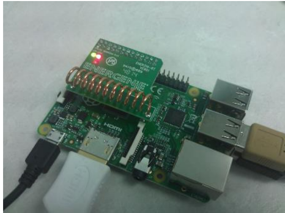
Figure 1 (Raspberry Pi B+ with RF Transceiver Board)
