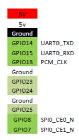
Figure 2 (GPIO pin header)
