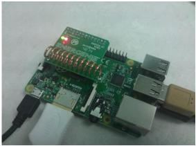
Figure 1 (Raspberry Pi B+ with RF Transceiver Board)
