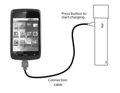
1. Connect the charger to your mobile device using the cable supplied or use your own USB cable.
